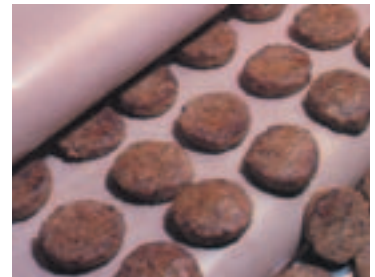
Continuous double-sided grilling of sausage patties
