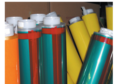
Pressure sensitive tape logs secured against unwind
