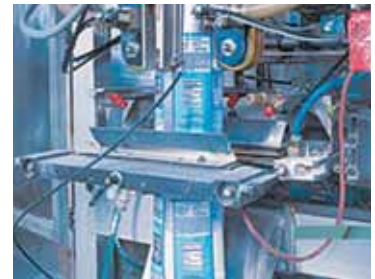
Plastic bag seamed and sealed by VFFS machinery
