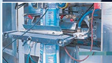
Plastic bags seamed and sealed by VFFS machinery
