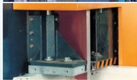
PVC extrusion welding, platen cover
