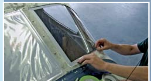
Plane paint masking
