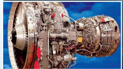
GE aircraft engine series CF6-80
