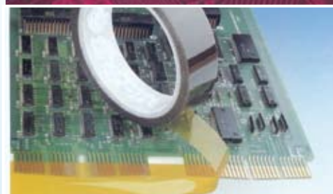
Finger masking with polyimide tape
